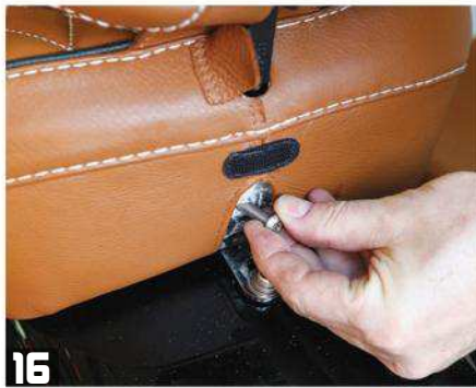
16 This is where the bolt installs to set and lock the backrest in place. Again, we have the flap up and out of the way to better show how this works.
