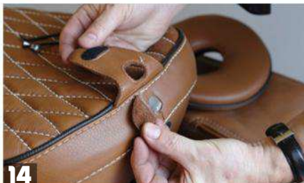
14 Move the top flap and then the side flap away to access the mounting areas for the rear backrest.
