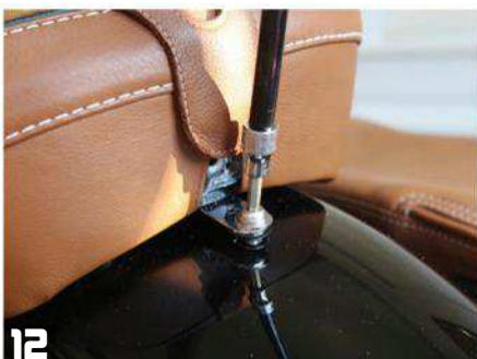
12 Once the new saddle is held in place up front, reattach the rear mounting bolt with the plastic washer between the painted fender and the metal mounting tab. The Corbin saddle does not use the left- or right-side factory mounting bolts.
