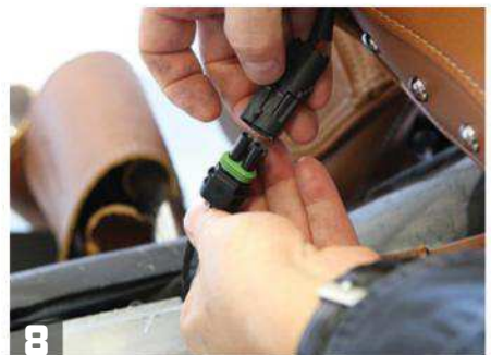
8 Note the connected wire harness from the stock Indian electric heating. Disconnect it, as you will need this for the new Corbin saddle.
