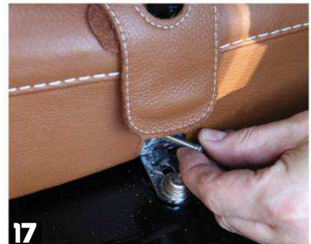
17 Flap down for final installment, this is where the bolt installs with the supplied Allen wrench to lock everything in place.
