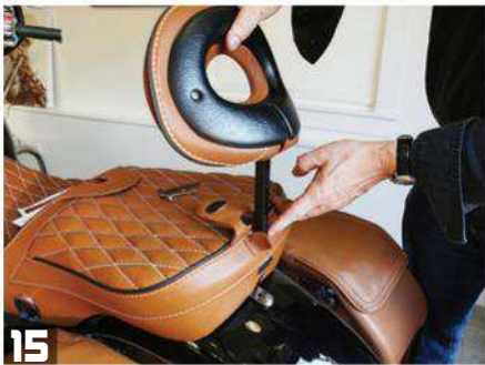
15 We pulled back the leather cover to show more clearly how the backrest installs into the rear of the saddle. The final install is with the flap down for a cleaner look.
