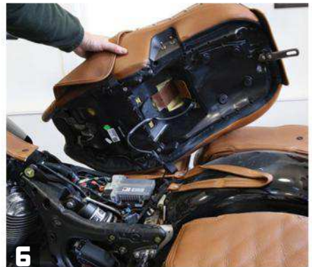
6 Having removed the two side mounting bolts and one rear one, carefully lift the back of the saddle and gently pull it back and up to remove the stock saddle.
