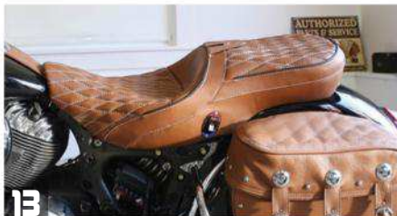
13 The Indian Roadmaster Classic with Corbin saddle installed. It looks very much like the stock one, but it's slightly wider and heavier due to the cooling system under the base plate.
