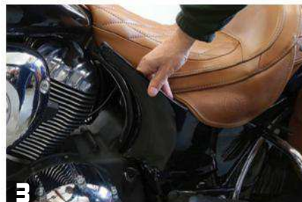
3 Remove the stock pop-off side covers and put them somewhere safe where they can't get scratched or otherwise damaged.
