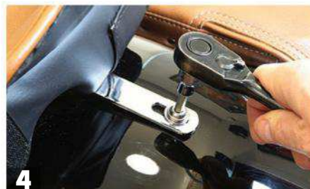
4 Use a 6mm Allen wrench to remove the stock bolt holding down the rear of the stock saddle.
