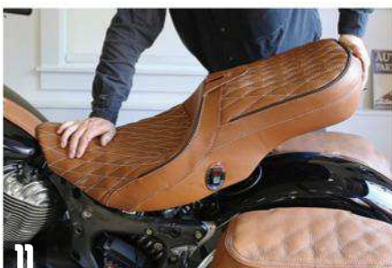
11 Installing the new Corbin saddle for the first time takes some patience. You need to slide the front of the saddle down and under the mounting brackets up front. It took me a few tries to get it, but once in, it fits snugly.
