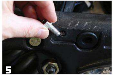
5 Use the 6mm Allen wrench to remove the stock side mounting bolts. There is one on the right and one on the left.
