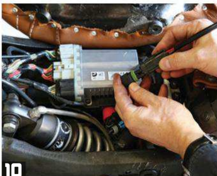
10 While balancing the new saddle on the bike, connect the stock wire harness from the bike to the new one on the Corbin saddle. They are designed to fit perfectly.
